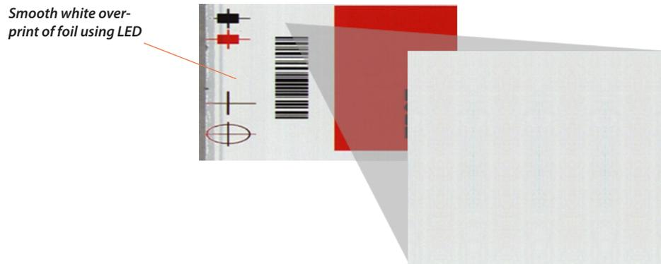
The magnified image shows how the white overprint appears smooth, visually accurate with no color distortion or compromise on inspection settings.
