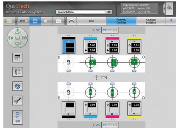
Automatically controls fan-out and cocking
