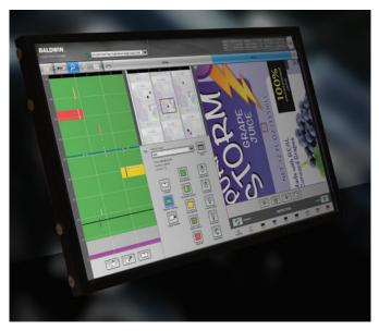
The Inspection System's live, color-coded roll map allows operators to quickly identify different types of defects, and make fast decisions about defect severity and remedy.
