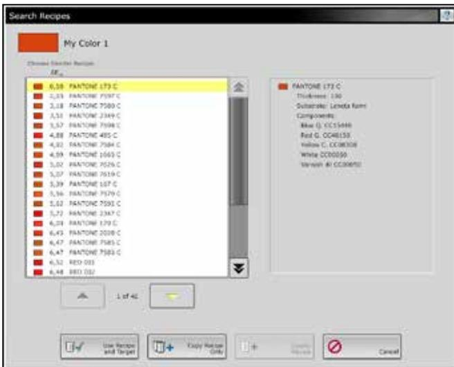
Ink waste can be reduced through the use of software tools that search a recipe database for the best match from previous printruns. Rather than making multiple batches from scratch, existing inventory can be repurposed. Photos courtesy of QuadTech
