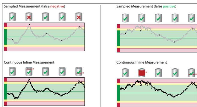
Sporadic sampled measurement gives an inaccurate picture of print performance, resulting in enormous waste—or worse, defective material being sent to the brand owner.
