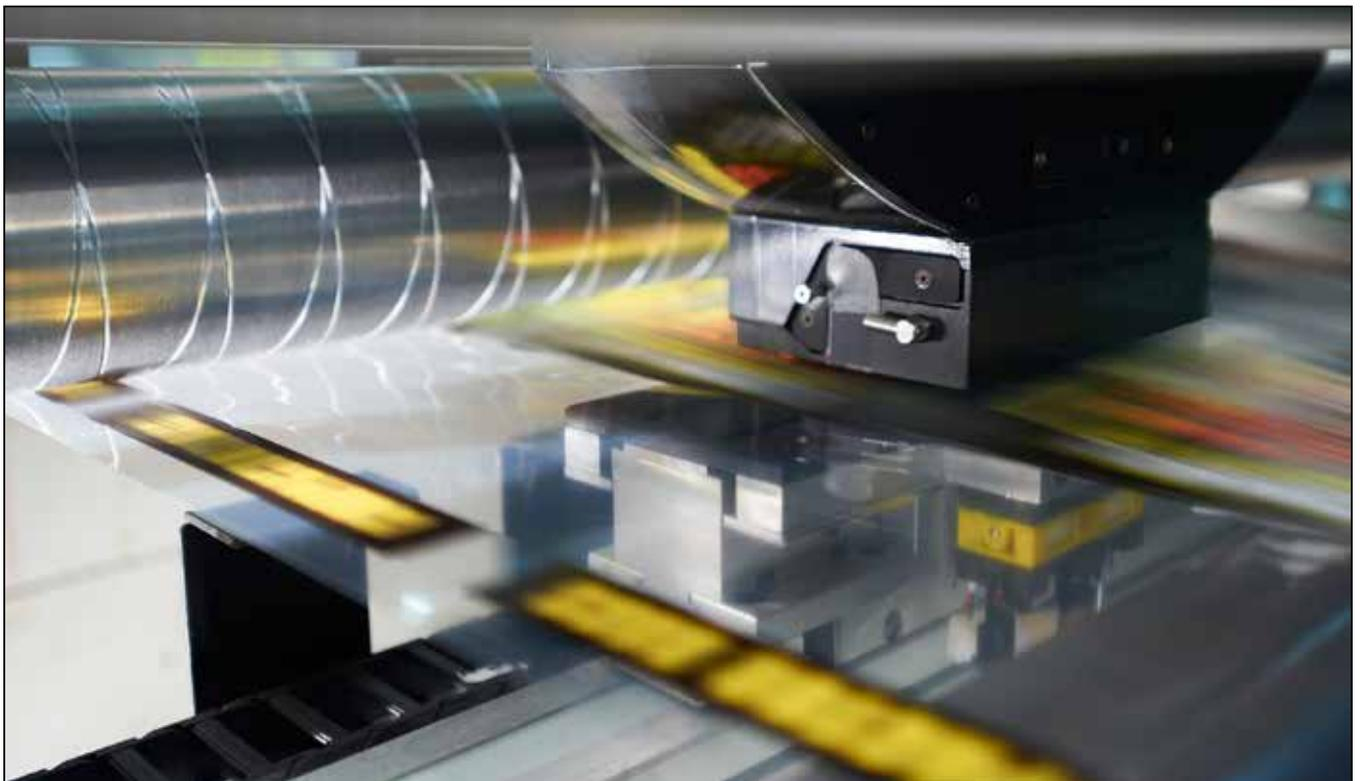
Exact recipe corrections can be calculated automatically and formulation software will tell the operator precisely how much ink needs to be added. Once this has been completed, the inline measurement system will provide immediate feedback on the success of the correction. Such a system could also manage and correct overprints, monitor ink consumption and calculate the correct mix for even the smallest volume.
